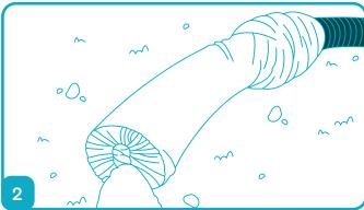
Thread the drainage pipe through the centre of the applicator and tie a temporary knot on the FilterSleeve to prevent it sliding back over the pipe end.
