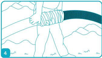
Holding the drainage pipe and applicator along the length of the pipe, maintain even tension on the FilterSleeve as you feed it to the other end for maximum yield.
