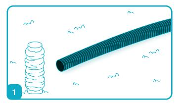
Ensure that the drainage pipe to be covered is uncoiled as much as possible, preferably alongside a pre-dug trench with your FilterSleeve ready to be applied.
