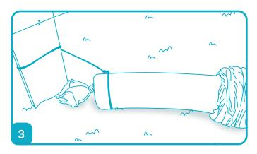
Secure the end of the pipe to an anchor point (e.g., post, tree, vehicle, etc...)
