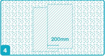
If you are connecting two pieces, then that the fabric is spread out with no wrinkles, then ensure to maintain at least a 200mm overlap between the pieces.
