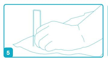
Pin the fabric on a slope or trench, with spacing that suits the application. We recommend using Strol Weedmat Pins or SquarePegs to secure your SureTex Geotextile in place.
