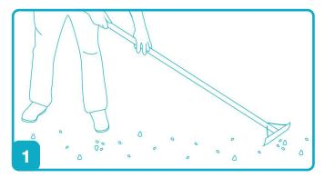
Prepare the ground by clearing away any rocks and debris, then level as much as possible to ensure the SureTex Geotextile will have adequate ground contact.
