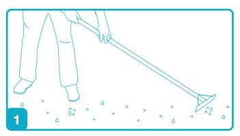
Prepare the ground by clearing away any rocks and debris, then level as much as possible to ensure the SureTex Geotextile will have adequate ground contact.
