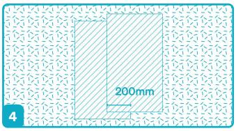
If you are connecting two pieces, then that the fabric is spread out with no wrinkles, then ensure to maintain at least a 200mm overlap between the pieces.
