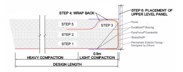
Once the backfill elevation at the face has reached 600mm compacted depth, pull the facing wrap from the front of the panel back over the compacted soil. Pull the facing wrap taut. It may be necessary to stake or pin the wrap to keep it taut while backfilling. Continue the construction sequence by placing another row of DuraMesh<sup>®</sup> panels and repeating the construction steps (refer to the figure above for correct placement).
