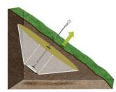
The third stage is where the anchor produces its ultimate load. As the anchor load approaches the bearing capacity of the soil, the rate of increase in load will reduce until bearing capacity failure of the soil takes place.
