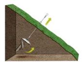
The first stage is where a load is applied to rotate the anchor into its loadlocked position. Elements of both load and extension are present.
