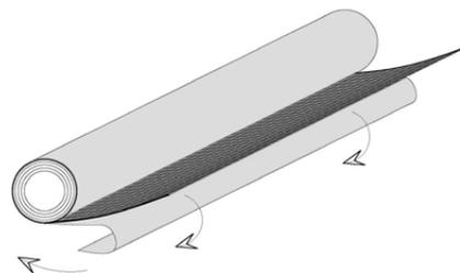
4. Pull release film upwards and unroll HaTelit® BL in direction of laying while gently tautening. Finally press down sheet using broom or small roller.
