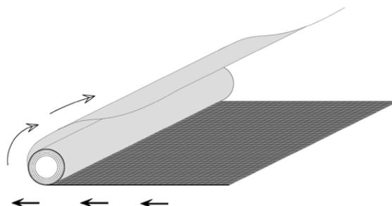
5. Sheet can be carefully cut off from roll with sharp knife at end of laying section.
