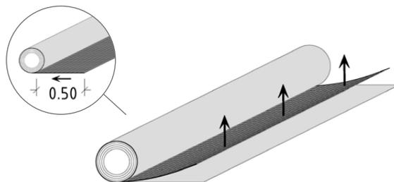
3. Fold back peeled release film under roll and apply exposed bitumen backing to base. Slightly press down contact surface of HaTelit® BL and then roll sheet back.
