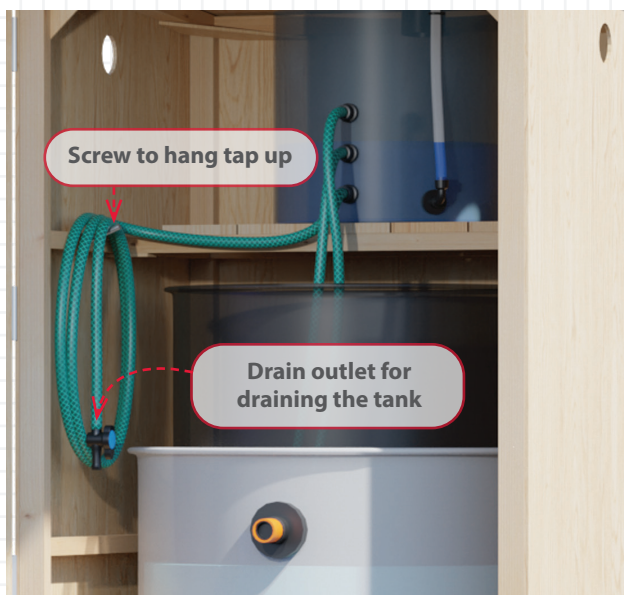
Fig. 1.9 Drain tap detail (Ensure remains closed during operation)
