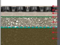
Fill SurePave (STEP 9) SurePave (STEP 7) Bedding Layer (STEP 6) Geotextile - optional (STEP 4) Base Course (STEP 3) Geogrid - optional (STEP 2) Geotextile - required (STEP 2)
