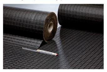
In the cross direction the overlap should be 150 mm. When placing several roll widths side by side the joints should be staggered. The overlaps should be treated with a minimum of  $0.15~{\rm kg/m^2}$  of bitumen emulsion.
