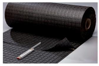
In the length direction the jointing of the rolls should be with a 250 mm overlap. The end of a roll should always be placed over the beginning of the next, ensuring the overlap is not lifted during the asphalt covering operation.
