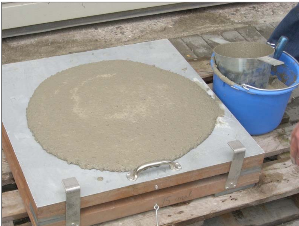
Illustration 1: Determining the slump acc. DIN EN 12350-5
