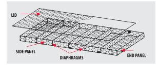
Assemble each mattress individually by raising the sides, ends and diaphragms. The various elements of a mattress are shown in sketch above.
