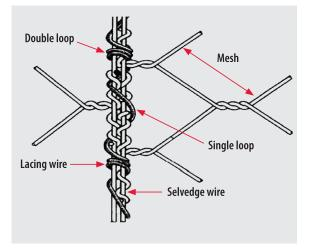
wire around the selvedges, then lacing around the two edges being joined, using a double tie through each mesh in turn, and tie off securely at the bottom, see sketch above.
