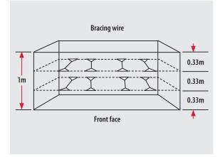
Provide internal horizontal bracing wire at 0.33m vertical centres in 1 m deep gabions, at the ratio of four wires per cubic metre, see sketch above.
