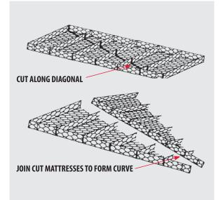
Mattresses can be cut and folded to form mitre joints and non-rectangular shapes. The mesh must be cleanly cut, and the surplus mesh cut out or folded back and neatly wired to an adjacent mattress face.
