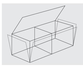
First lace the four corners of the gabion, then the diaphragms to the sides. Always begin lacing at the top, twisting the end of the lacing
