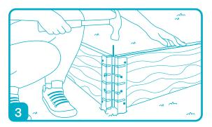
Make sure that the two sides are properly aligned, then hammer one of the pins provided into the hole connecting the joining brackets to secure the sides.
