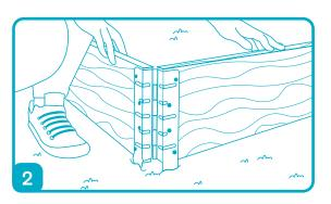
To begin creating your GardenStax, simply connect two sides together by aligning their joining brackets.
